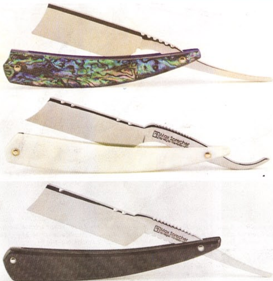
Three handcrafted straight razors by Max Sprecher of Las Vegas. At top, 15/16" wide "Spanish Point," quarter hollow ground, with extra long tail and scales of blue paua shell laminate. Middle razor is a wedge ground 13/16" "Humpback" handled in faux ivory G10 fiberglass. At bottom is another "Humpback" in a 7/8" width, quarter hollow ground, with carbon fiber scales.
